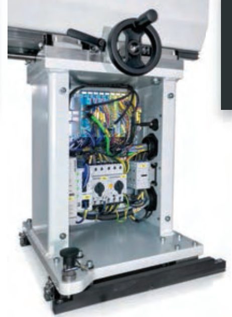
The robust, compact and modular "S-DIAS" control and I/O modules from SIGMATEK fit directly in the brush robot stand.
