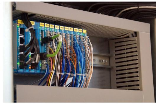
The compact »S-DIAS« control system from SIGMATEK operates the entire regulating technology of the dosing system, as well as recipe management.
