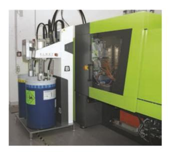
Through the new, open construction of the »Top 5000 P $\alpha$  dosing system, the containers can now be comfortably exchanged from the front and side.
