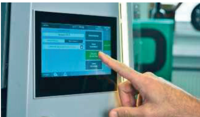
Central element of the control technology: Operating Panel ETT 732 with a 7-inch dual-touch TFT color display and EDGE2 Technology processor.
