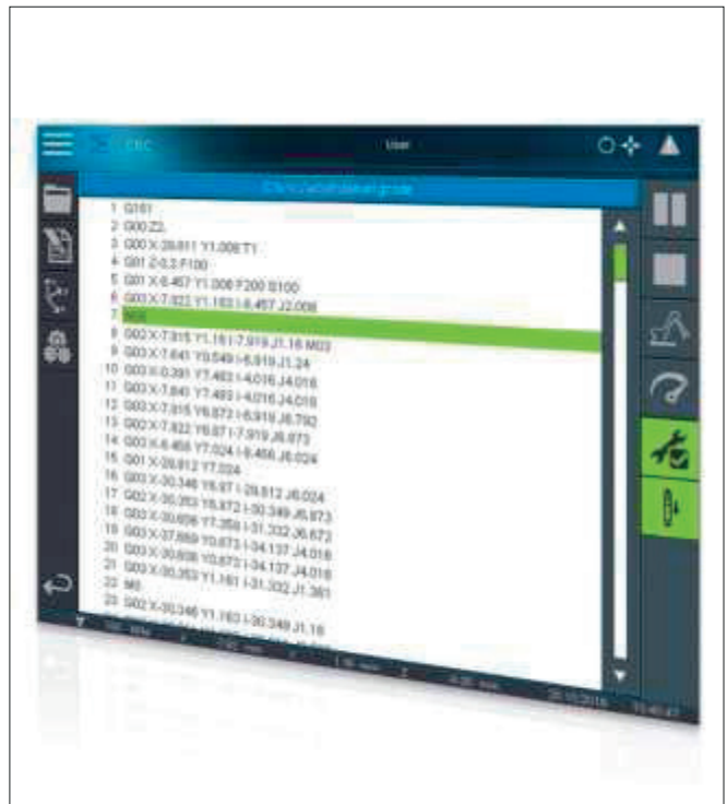
The G-code interpreter is a component of the engineering environment LASAL and was expanded with the sequential processing of large programs.
