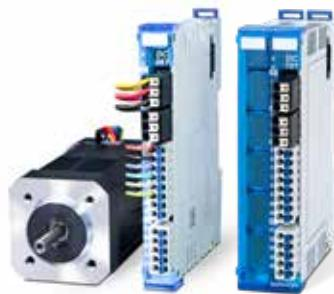
With the DC 061/101 (resolver) and DC 062/102 axis modules (incremental encoder), full servo functionality is provided in DIN rail format. The power output stages are embedded in the S-DIAS control and I/O system, and provide 300 – 480 Watts of rated power, a 2-channel enable input for implementing STO, as well as a +24 V DC output for controlling a holding brake.
