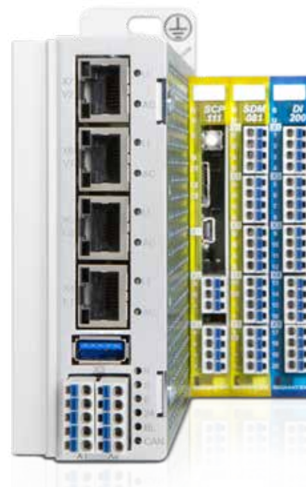
The CP 731 and the CP 733 with powerful Intel® Atom™ dual-core processor.
