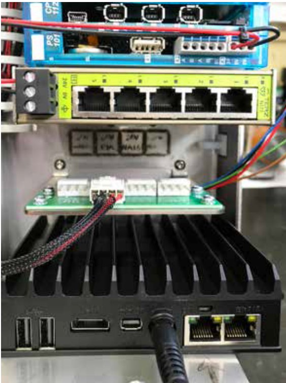
SIGMATEK SlamLoc is optimized for operation in 64-bit industrial pc and is also provided by SIGMATEK as a bundle, including the hardware with WLAN connection (below).
