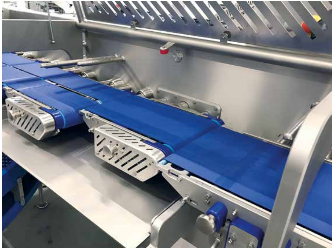
In the “lane divider”, the stacked burgers are placed in the correct configuration and alignment.
