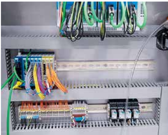
The modular DIAS Drives 100 from SIGMATEK control the servo motors and communicate with for example, SinCos interfaces. In this configuration, transport and conveyor belts are controlled. In combination with the Ethernet bus system, the S-DIAS control system with integrated Safety ensures data communication in hard real time.
