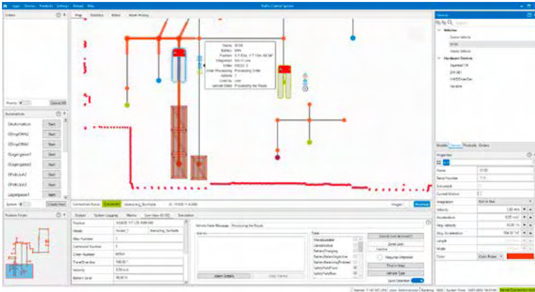
The visualization shows permanent, real-time display of the location, direction of movement, speed and battery power status of the individual vehicles
