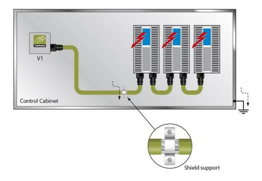
If two control cabinets must be connected over a VARAN bus, it is recommended that the shielding be located at the entry points of each cabinet. Noise is therefore prevented from reaching the electronic components in both cabinets.
