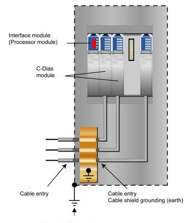
The control box must be connected to earth!
