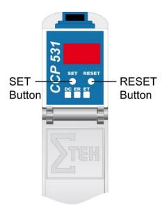
To enter the mode for setting changes, press and hold the SET button while the C-IPC is booting.
