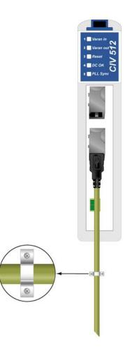
The VARAN cable should be secured against vibrations with a distance of 20 cm from the connector (for example with a clamp)!
