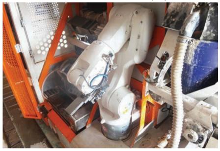
Insight into the "Pax" masonry robot: at the bottom left is the sawing unit, next to it the robot that lays bricks as well as applies mortar, on the right the cement pumping unit and the mortar supply hose.
