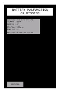
Information on the defect of the battery indicated can be read from the log files.
