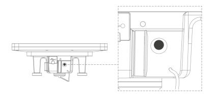
The operating panel is equipped with an alarm signal (Piezzo). To avoid minimizing the specified volume, the sound outlet must be kept free of obstacles (finger...).
