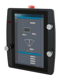
In combination with a BWH 001 base station and a safety-related PLC, the HGW 1033-32 is a wireless, intelligent manual operating unit with emergency stop function that enables the programming, visualization and diagnosis of processes and systems control.
