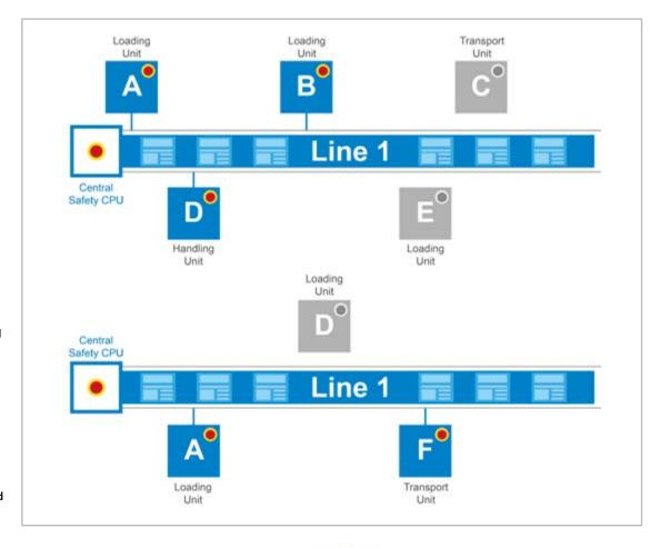
Typical example application from the plastic and paper packaging line: The modular loading and unloading units, as well as handling and transport systems with emergency stop function, can be integrated into or separated from the line as required via S-DIAS Safety's Hot-Swap feature during operation and without a hardware switch.
