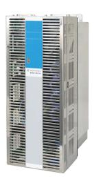
The SDD 215 is a 2-axis unit designed for midrange power applications. One axis can operate with 10 A continuous and 20 A peak current, the other with 15 A nominal and 30 A peak current. This allows a varying number of axes as well as motor combinations with different capacity ranges to be implemented.
