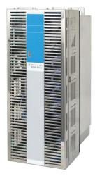
The SDD 315 is designed for midrange power. With this three-axis drive, one axis can be operated with 15 A continuous and 30 A peak current. The others are operated with 10 A nominal and 20 A peak current. Motors with different power ranges can therefore be combined.
