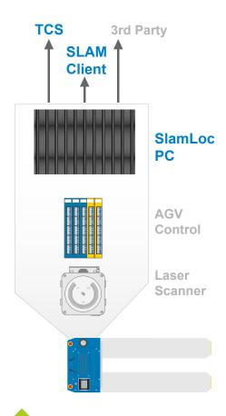
SIGMATEK SlamLoc can be used as a pure software solution or preinstalled in robust Mini-PC. With SlamClient, the actual vehicle movement can be visualized.
