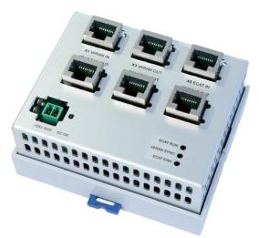
The VARAN Out ports have automatic Ethernet recognition. If one of the ports is connected to an Ethernet participant, it automatically becomes an Ethernet port.
