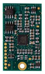
The VEB 011 VARAN client board serves to easily expand all possible peripheral devices with the VARAN bus. Operating temperature 0-70  $^{\circ}$ C (commercial grade).
