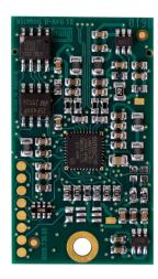
The VEB 011C VARAN client board serves to easily expand all possible peripheral devices with the VARAN bus.
