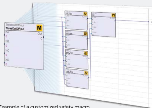
Example of a customized safety macro that evaluates several input signals in relation to each other and generates a corresponding output signal. Such macros can then be used as often as required in the safety application.
