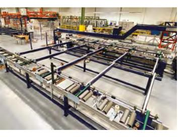
The Swiss machine builder Müller TB builds equipment for the fully automated processing of aluminum frames for window production.
