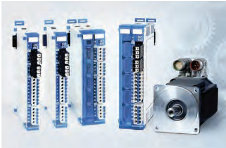
Compact SIGMATEK DIN rail modules for motor control: DC series for servomotors, SR series for DC brush motors, ST series for stepper motors.
