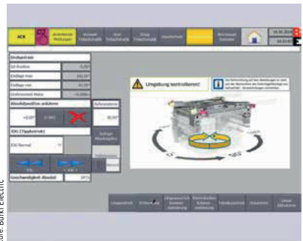
Each axis can be moved individually during service operation.
