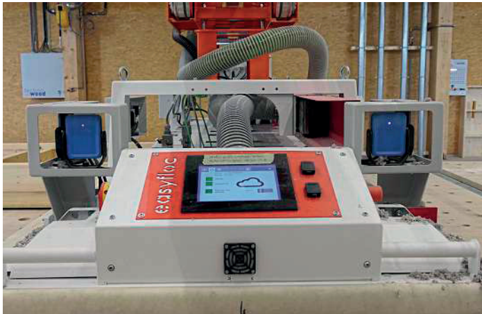
The 8-inch multi-touch ETV 833-3 operating panel is installed directly on the G3 blow-in plate.
