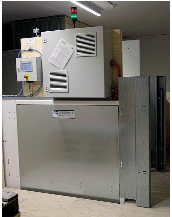
Control cabinet of the injection module with the compact 7-inch operating panel from SIGMATEK.
