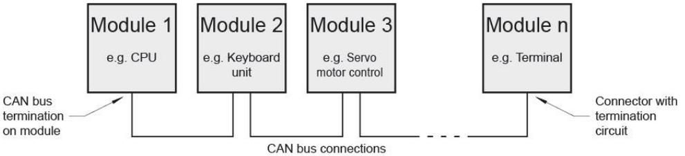
**The termination is made by an internal 120  $\Omega$  resistor between CAN A (LOW) and CAN B (HIGH).**
