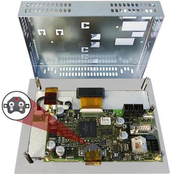
5. Using the strap, remove the battery from the holder.
