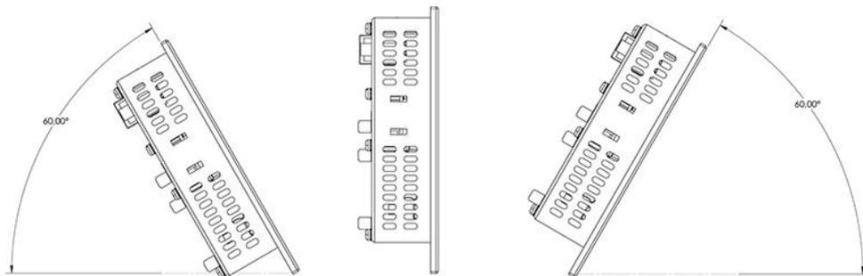
The screw-mounted brackets can be tightened with a torque of 0.15-0.20 Nm. For this purpose, a 3 x 0.5 flat-tip screwdriver is required.
