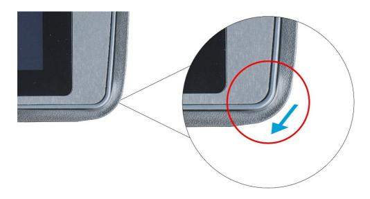
3) Ensure that rim of the edge protector lays flat on the handheld operating panel.
