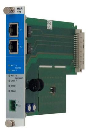
With this module, the VARAN plugs and the power plug are connected to the front panel. In addition, the interface module has an inrush current limiter. To avoid misplugging, a DIN connector (connection to the module carrier) is offset from I/O base or fan module.
