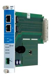
With this module, the VARAN bus and the power plug are connected to the front panel. In addition, the interface module has an inrush current limiter. To avoid misplugging, a DIN connector (connection to the module carrier) is offset from I/O base or fan module.
