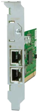
The PCI insert module, PVC 531 with integrated VEB 031, can be used in any standard PC. A VARAN Manager is available on the PC and serves as an interface between the PC and VARAN bus.
