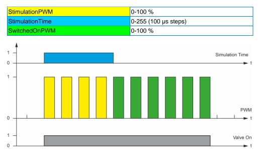
These setting parameters make it possible to control the valve as energy-saving as possible.
