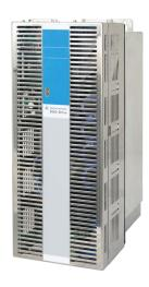
The SDD 335 is designed for high power. With this three-axis drive, one axis can be operated with 10 A continuous and 20 A peak current, one axis can be operated with 10 A continuous 30 A peak current and one axis can be operated with 15 A continuous and 35 A peak current. Motors with different power ranges can therefore be combined.
