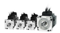
The low-voltage synchronous servomotors from the SM series are brushless, rotary current motors with have permanent magnets in the rotor and threephase windings for special servo applications. The neodymium magnet material and the low inertial moment contribute significantly to making these motors highly dynamic and allow them to have a very low cogging. The robust and compact motor with high power density is available in three performance classes 60, 100 and 200 watts.
