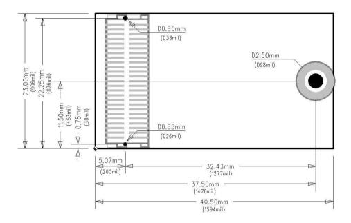
The dimensioning of the center holes of the 50-pole ERNI Board-to-Board connector is effective for the plugs on the base board (doesn't show the position of the connectors on the VEB).
