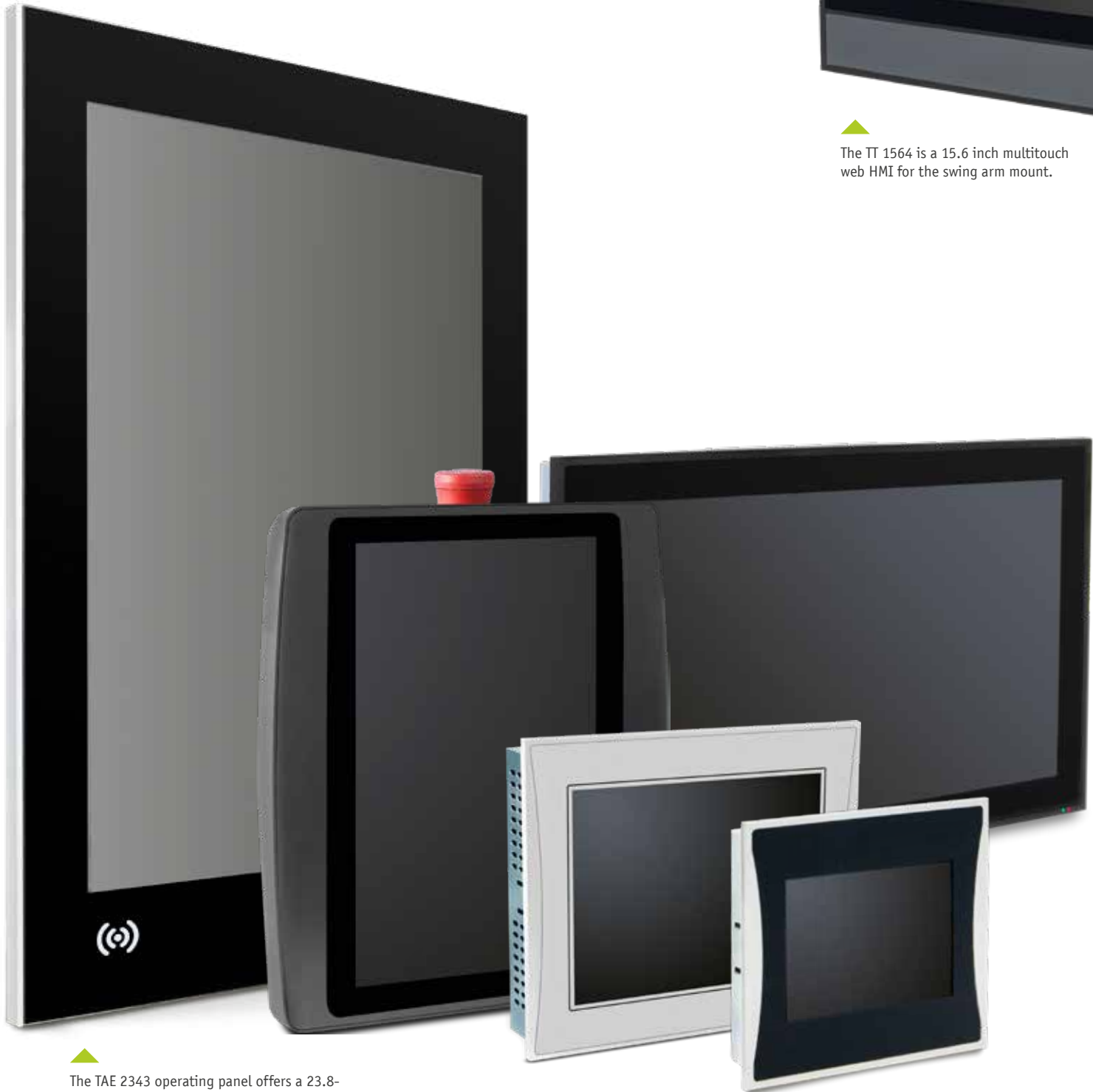
▲ Small panels for operating and monitoring are already available from 3.5 inches - here the ETT 312.
