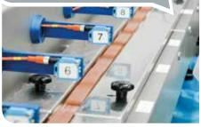
Customer specific conveyor and feeder systems: up to 500 units per minute - several highly dynamic motion axes - synchronization of the servo motors in hard real time with the industrial Ethernet VARAN.
