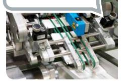
The friction feeder "Motion Feeder" operates with up to 800 cycles per minute – flat products such as package slips for medication are therewith separated, counted and in a package, also position-synchronized servo drive controllable up to 240 m/min.
