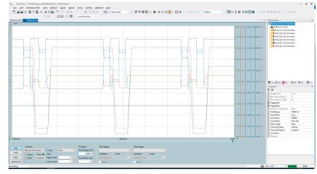
In the diagnostic tool of the LASAL design environment, the axis positions (e.g. of the robot) can be precisely tracked and deviations detected.
