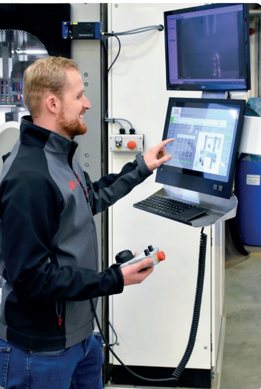
Operation and monitoring of the additive manufacturing systems are performed via visualization created in LASAL on a TT 1933-S multitouch operating panel from SIGMATEK with 18.5" WXGA TFT color display.
