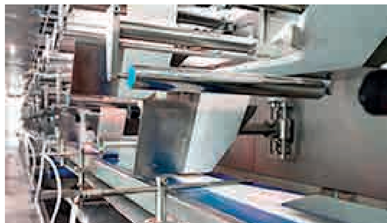
► The damp fabric panels are brought into position over one another. Rotating blades cut the fabric to the desired length (600 cuts/min).
