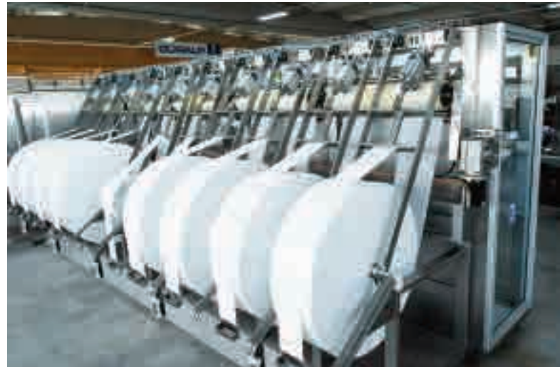
► Between 10 and 24 fleece rolls are used for wet wipe processing.
