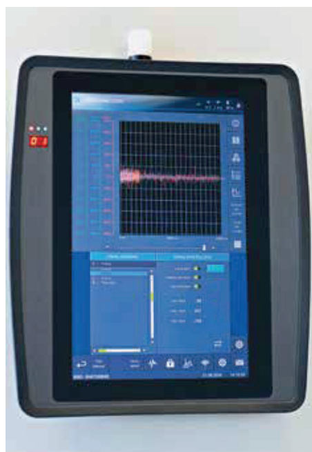
The wireless panel's oscilloscope function allows the operator to monitor a signal in real time to detect any anomalies.
